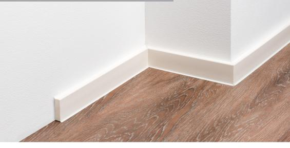
If nailing, galvanised steel nails must be used. The required length of the nails depends on the existing substrate. The distance between the nails should be between 25 and max. approx. 50 cm. The nails are to be arranged with an offset.
