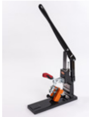
ARTICLE 22251 BOLTA-SL punch for 5mm profiles
